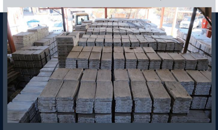
Over 60,000 meters drilled and sampled. Main core storage at Cuchara site
